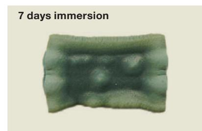
The above picture and graph are based on our experiments, and they are reference data. Hydrotite CJ starts to swell from its edge / corners partially and continues to swell gradually overall.
